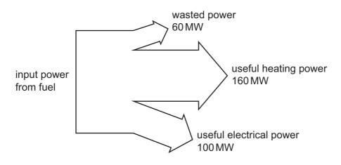
What is the efficiency of the CHP station for producing useful power?
