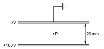
What is the electric field strength at point P midway between the plates?
