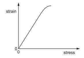
Why is the strain energy per unit volume of the material not the area under the graph?
